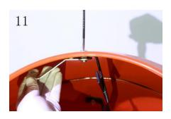
Assemble the mixing blade with tools
