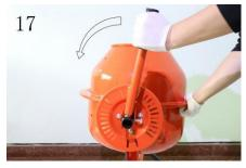
Press the drum with right hand, push With your lift hand toward the arrow. To make the screw into the hole.
