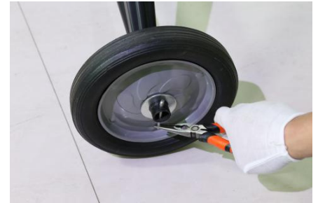
Fix the wheels on wheel bracket with tools.
